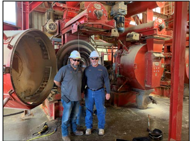
Woodville Pellet Plant Manager Bryan Davis and Production Manager Raul Pecina stand in front of one of the 12 machines that churn out the pellets via a 1,600-lb die that spins at 900 rpms.
